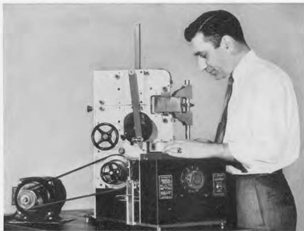
Figure 1. New Type 1700-B Variac Speed Control installed on toroidal winding machine.
